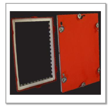
Fire Resistant Tab Access Doors meet the requirement of HVCA DW144 specification regarding air leakage criteria. These doors have been included in Fire Duct tests for fire resistance in accordance with BS 476 Part 24:1987, and have been assessed by the BRE Centre for Fire Resistance, as suitable for incorporation into a fire resistant ductwork system for periods of up to 2 hours Stability & Integrity.
